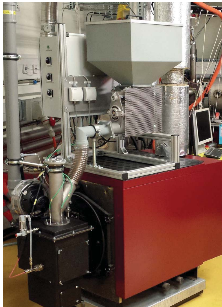
Retrofit wood gas burner (black) attached to standard fossil boiler (red)
