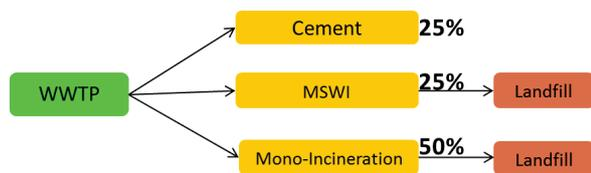
Fig. 2 – Present material flow of sewage sludge from WWTP [WWTP = Wastewater Treatment Plant, MSWI = Municipal Solid Waste Incineration]<sup>[3]</sup>
