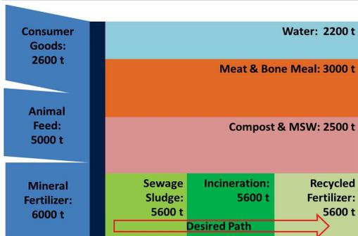
Fig. 1 – The flow of Phosphorus in Switzerland and potential recovery route [MSW = Municipal Solid Waste]<sup>[3,4]</sup>
