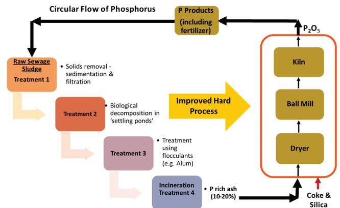
Fig. 3 – Proposed Closed Loop Model for recovery and utility of P from Sewage Sludge
