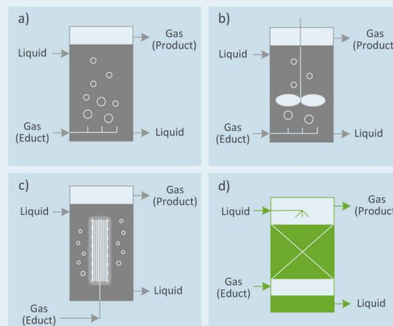
Fig. 2 Bioreactor types investigated for ex-situ biological methanation
