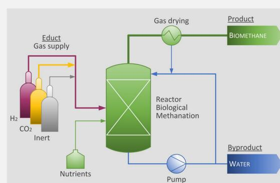
Fig. 3 Process flow diagram of biological methanation pilot plant at ZHAW
