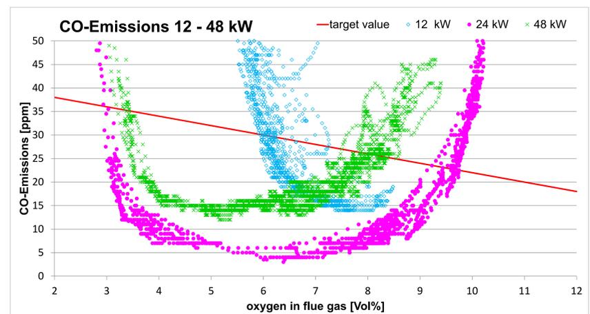
Figure 3: CO-Emissions as function of the oxygen in flue gas for different power
