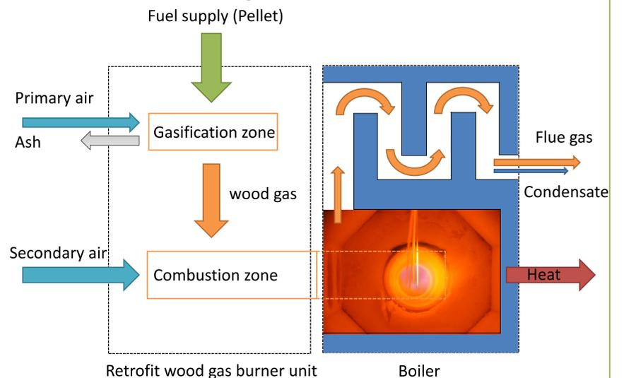
Figure 2: Process scheme of low emission staged combustion burner system
