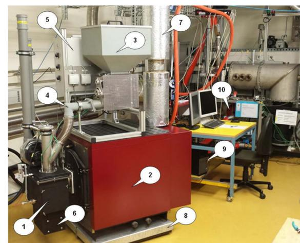
Figure 4: Retrofit wood gas burner (black) attached to standard fossil boiler (red)
