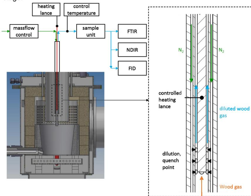
Figure 1: concept of the wood gas analysis
