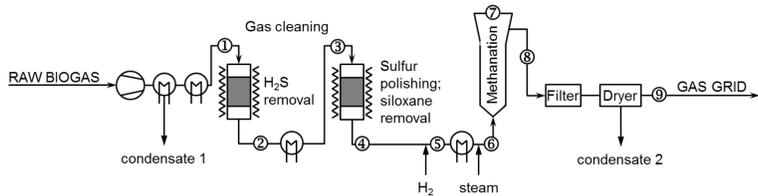
Because the methanation catalyst is sensitive to many biogas contaminants, especially sulfur compounds, specialized gas cleaning is needed. A two-stage gas cleaning process based on commercial sorbents is used. Gas quality is monitored by microGC, GC-SCD/FID, and Dräger tubes.
