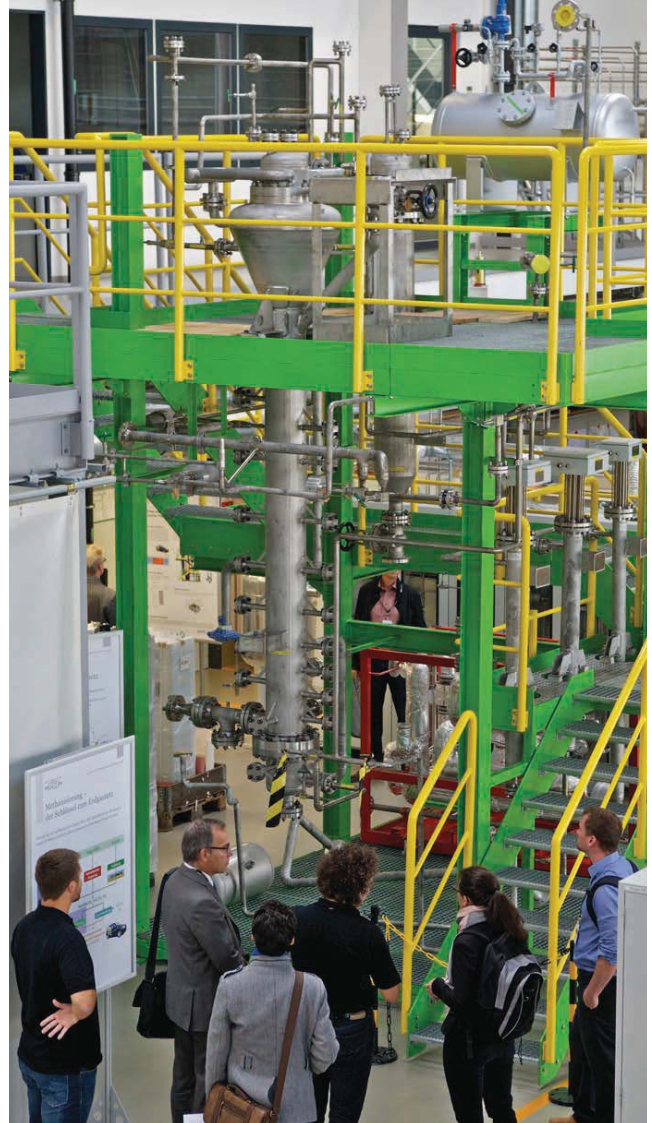
Catalytic methanation pilot reactor at the Paul Scherrer Institute
