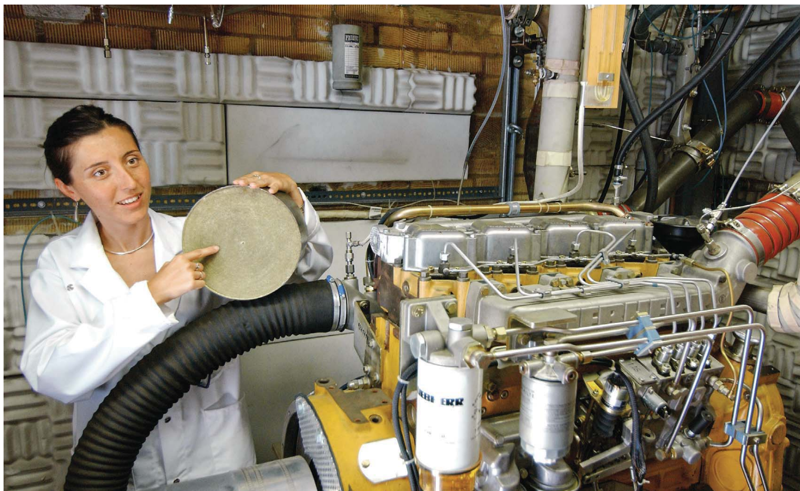
SCR catalyst at the Paul Scherrer Institute test facility
